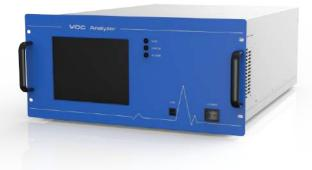
The EXPEC-2000 series VOC analyzer adopts three-valve four-column FID technology, which can measure methane, non-methane and BTEX simultaneously. This VOC instrument can be applied both in industrial emission and ambient air network round urban area.
