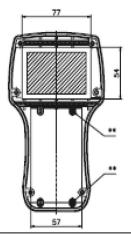
Free dimension tolerance to DIN 16901-130
